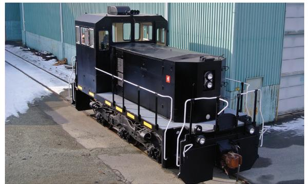
EMD D77 traction motors give a top speed of 40 km/h.
