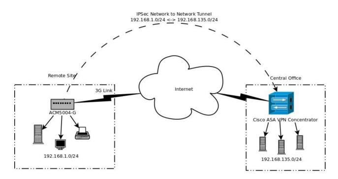
The ACM5004-G at the remote site has its Ethernet address set to be on the 192.168.1.0/24 subnet. It can either act as a gateway for that network, or simply be a member of the network. It is configured to initiate the IPSec connection. Please note that if the ACM is not the gateway, you must add a route to the router responsible for the network to forward traffic for the central office (192.168.135.0/24) via
