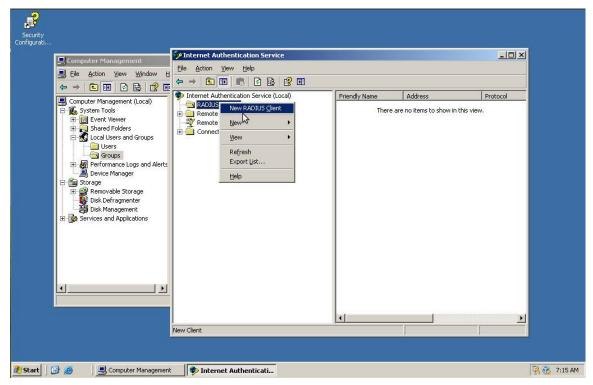
The RADIUS client corresponds with the Opengear device, so fill in the IP address or DNS name of the Opengear device, and choose a simple name for the device. This name will be used later on in the Remote Access Policy, so choose something consistent if you multiple devices.
