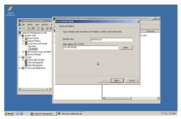
Now, choose a shared secret. This is the RADIUS password that is set on the Opengear device, and is used to encrypt all authentication traffic between the Opengear and the RADIUS server. Leave the "Request must contain Message Authenticator Attribute" tick box un-ticked.
